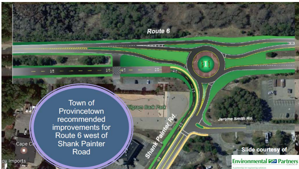
Concept plan of Town of Provincetown’s recommended improvements for Route 6 west of Shank Painter Road. A multi-use path is shown on the south side of the road.
