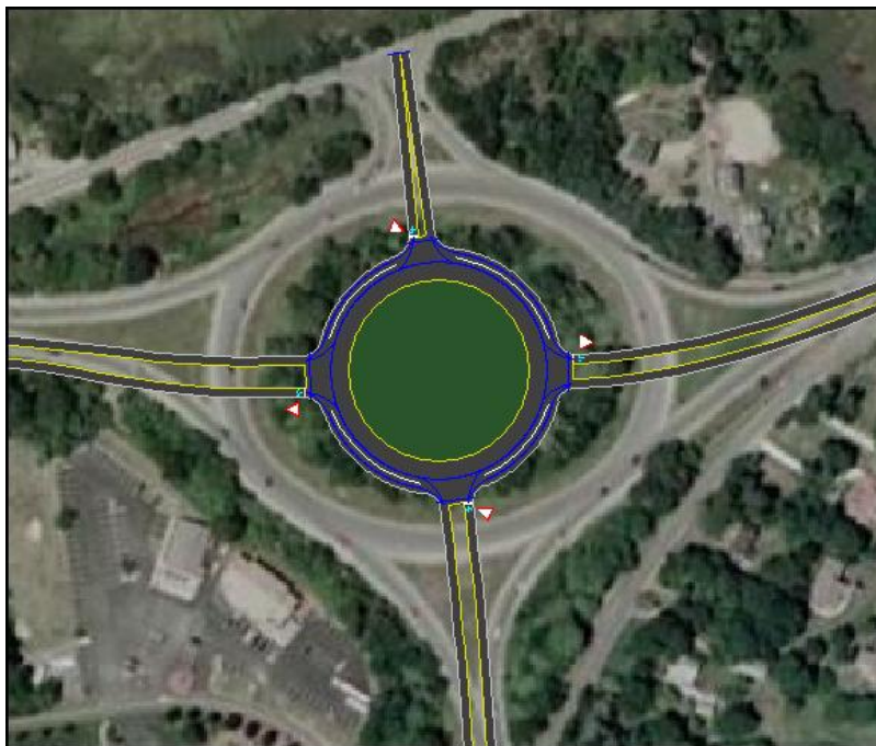
Figure 11 – Eastham Rotary, Modern Roundabout Alternative
